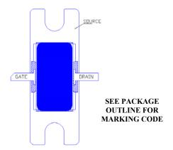
The FPD10000AF is a packaged depletion mode AlGaAs/InGaAs pseudomorphic High Electron Mobility Transistor (pHEMT), optimized for power applications in L-Band. The high power flangemount package has been optimized for low electrical parasitics and optimal heatsinking.
